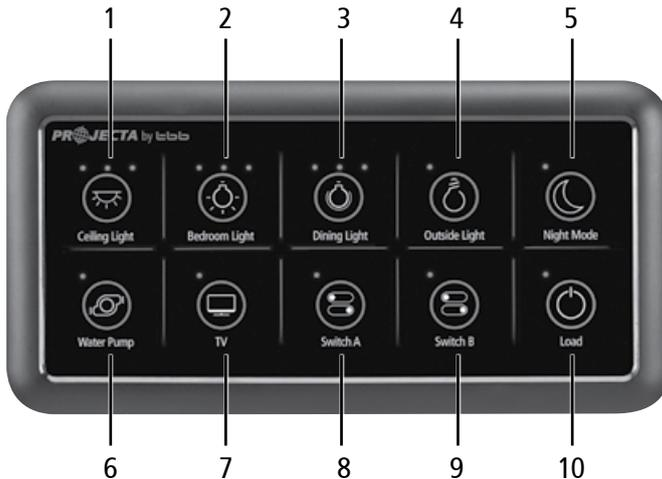
Figure 4 Overview of 10 Position Switch Panel PM4SW10
