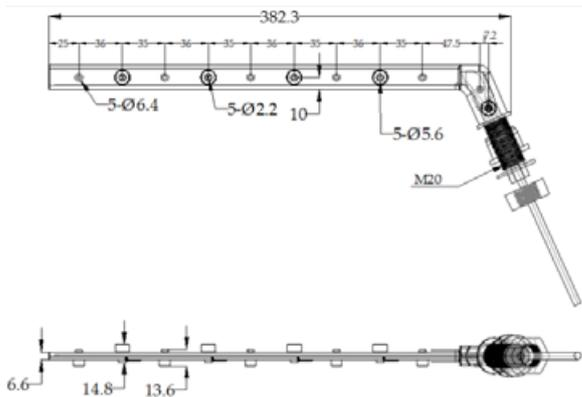
Figure 19 Dimension of PMWS400 (Unit: mm)
