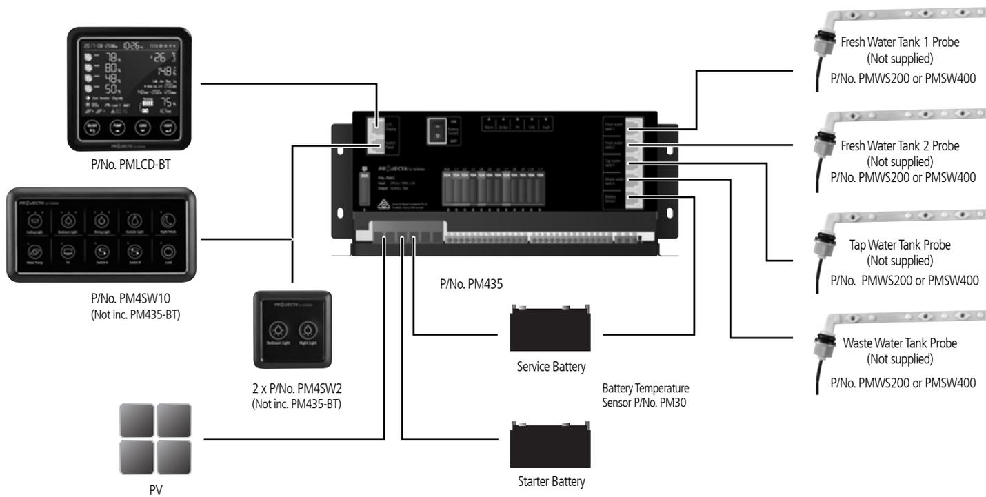
Figure 1 System Components for PM400 & PM435-BT
