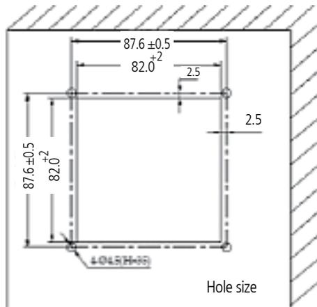
Figure 14 Installation of Monitor
