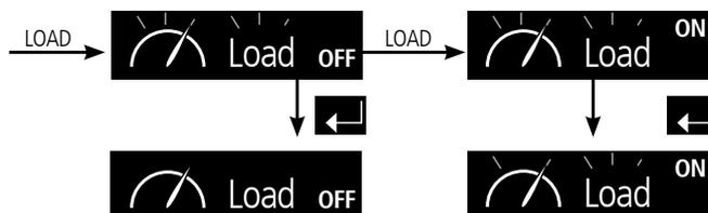
Figure 32 Switch ON/OFF all of the DC Loads
