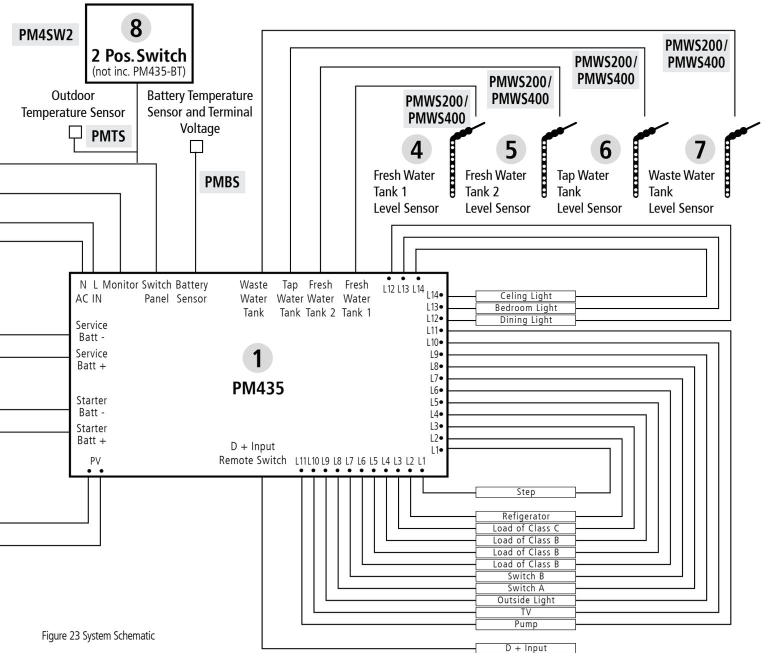
Figure 23 System Schematic
