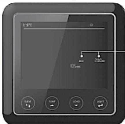
When the battery type and capacity setting on the monitor is not the same as PM435 dip switch, the icons are flashing.
