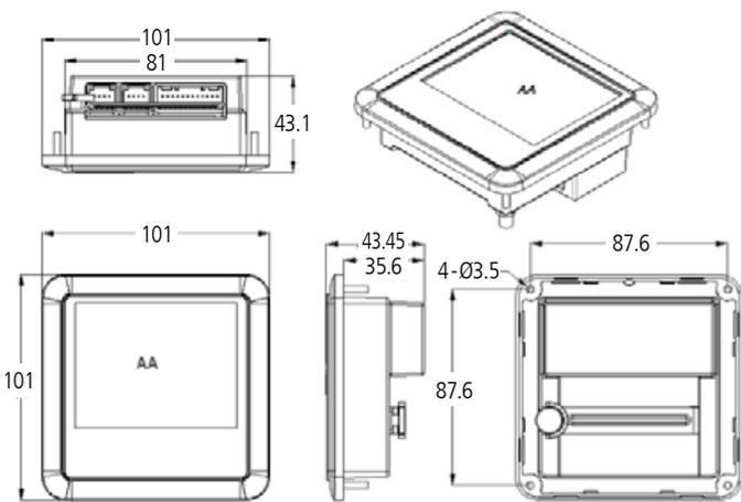
Figure 13 Dimension of Monitor
